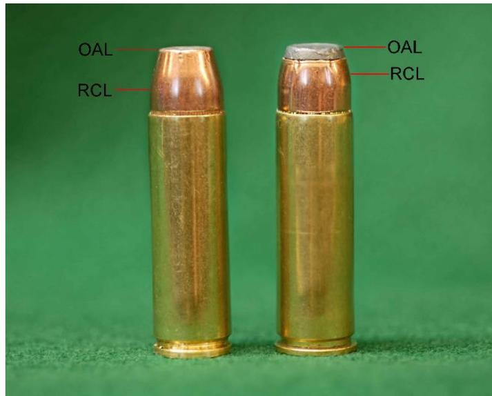
*OAL is the actual distance from the base to the very end of the bullet. RCL is the distance from the base to the working surface of the ogive of the bullet.*
