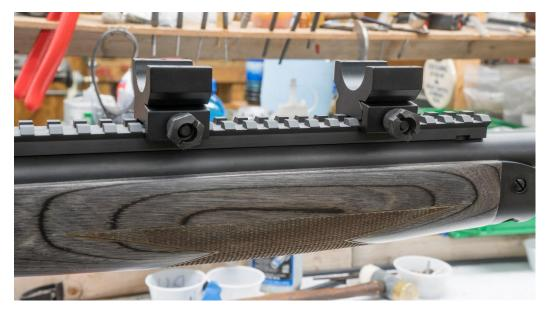
Put the scope in the rings, leaving the ring caps loose enough to slide the scope forward or back to adjust eye relief and rotate the scope to level the reticle.
