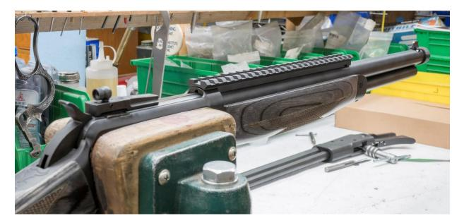
With your scout scope rail properly installed, now you can mount your optic. The Big Horn Armory Scout Scope Mount is made to Picatinny dimensions, so you can use either weaver style rings or Picatinny rings, whichever you prefer. Our scout scope mount is designed so you can use the iron sights when your scope is removed. We have used the Burris Xtreme rings and they have worked well for us.
