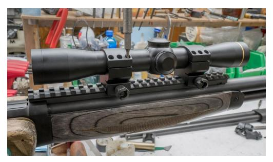
With your eye relief set, now level the reticle with the gun. This can be done just by looking through the scope and rotating it until it is level. You can also use a tool like Scope Jack from Fix It Stick, or a level to check the scope and rifle.
