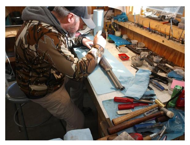
From there, the stocks are hand inletted and fitted to allow for glass bedding. All parts are coated with a release fluid and the epoxy glass bedding compound is applied as required. The whole assembly is then clamped together and left to cure overnight. Glass bedding enhances the durability of the wood-to-metal fit of our guns by creating a hard, smooth surface to interface with the metal. The epoxy will not allow the wood to compress in our high recoil firearms.
