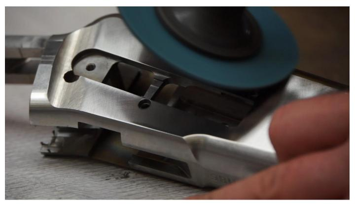
First, you start with polishing all the visible exterior parts. This is done to remove all machine tool marks. Then these parts are glass bead blasted in preparation for <u>salt bath nitriding (SBN)</u>. Barrels are ramped and chambers are polished to smooth, reliable cartridge feeding and extraction.
