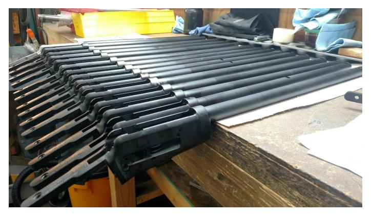
All of the parts are then gathered and assembly begins by mating the Magazine parts to the barreled Receiver. The Magazine Tube interior is polished and cleaned for smooth operation. It is also ground to fit since stacking tolerances between parts require fitting the oversize Magazine Tube.
