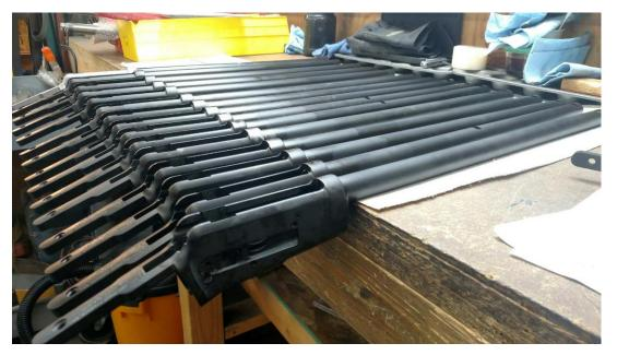
We heard about Salt Bath Nitriding (SBN) and the Quench/Polish/Quench (QPQ) procedure. Systematic nitriding has been around since the 1920s. Nitrogen and carbon are diffused into the surface of the steel, hardening it just like Color Case Hardening. It also turns the surface a uniform black when the QPQ process is used and leaves the original dimensions intact.
