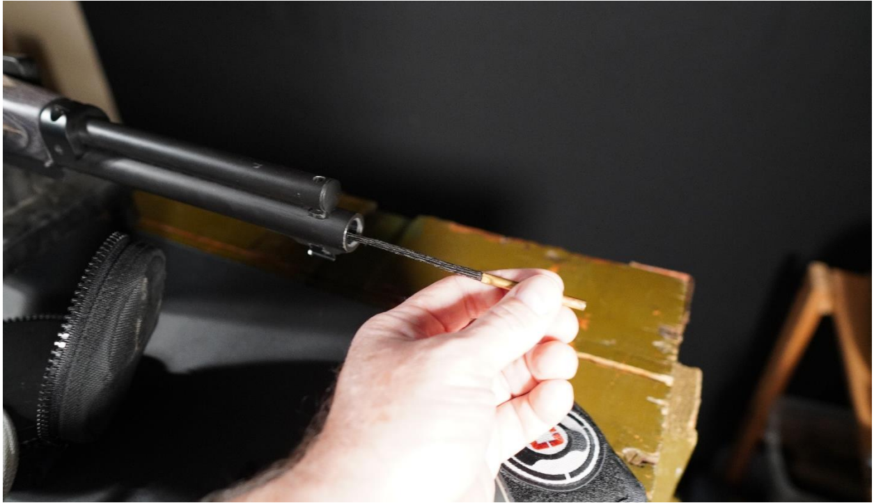
Pulling the Bore Snake straight through the bore to minimize contact with the crown/rifling.
