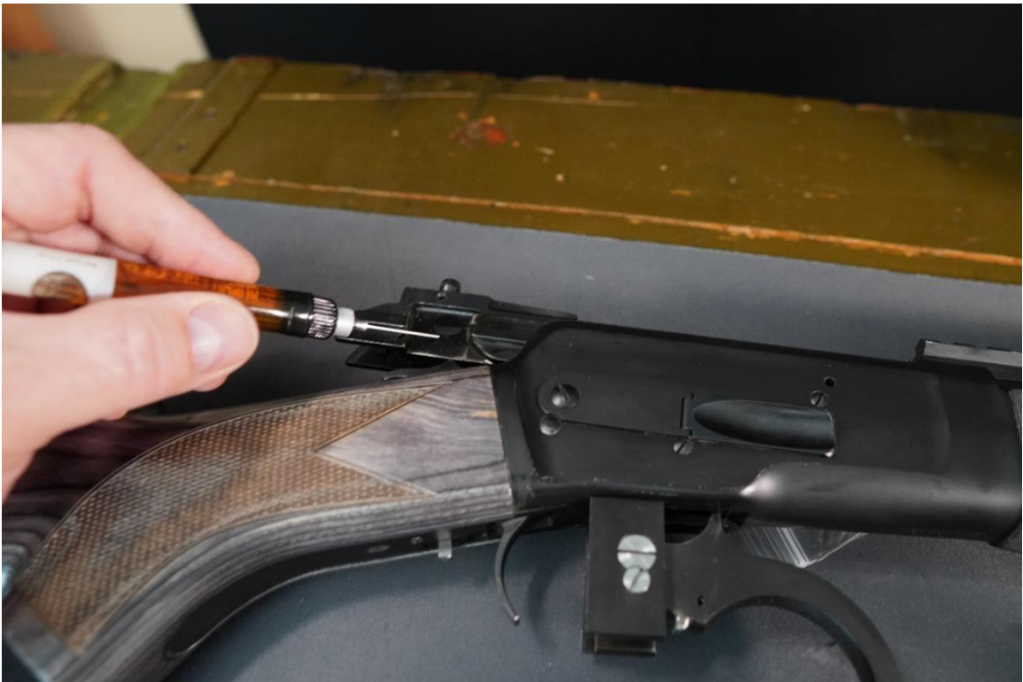
Apply a light coat of firearms lubricant to the moving parts of the action.
