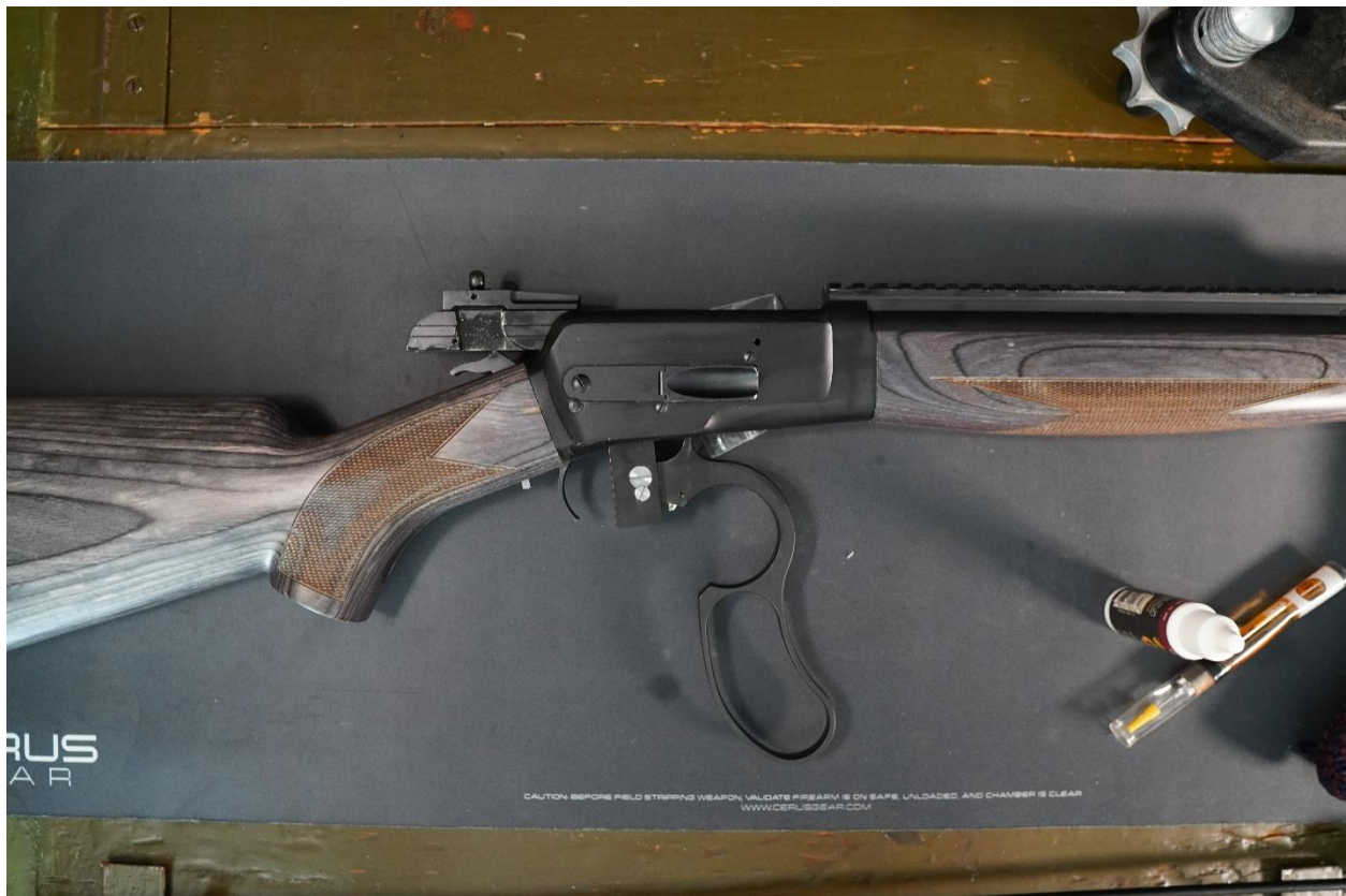
With the action open all critical parts can be cleaned and lubricated.
