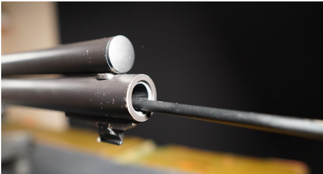
Notice how the rod contacts the crown/rifling. This is not recommended, particularly with steel or aluminum cleaning rods.
