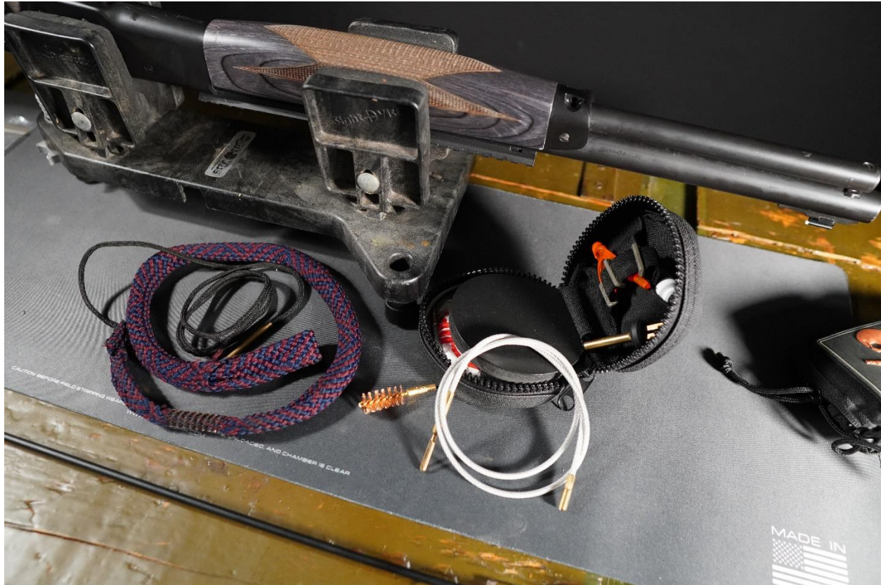
A “pull-through cleaning system,” like the Hoppes Bore Snake or Otis cleaning kit, are two styles of systems that let you clean from the breach-to-muzzle.
