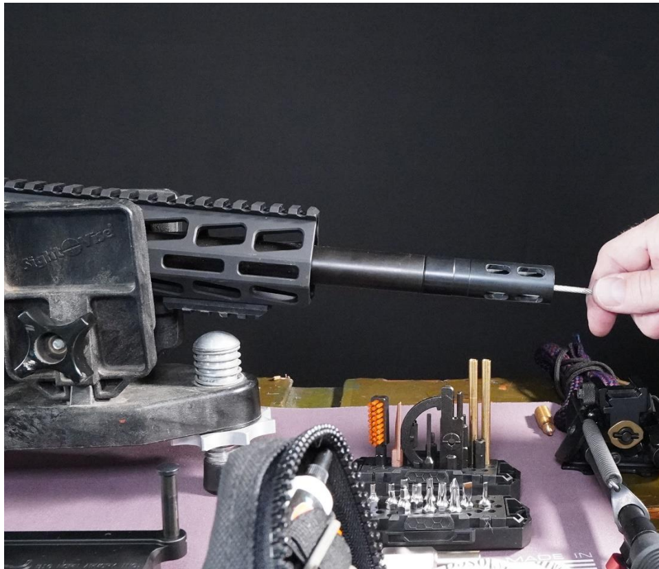
A "pull-through cleaning system" like the Hoppes Bore Snake or Otis cleaning kit are two styles of systems that let you clean from the breach-to-muzzle.
