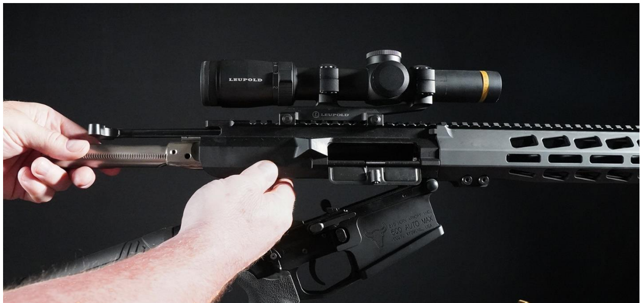
Separate the upper and lower receiver and remove the bolt assembly and charging handle.
