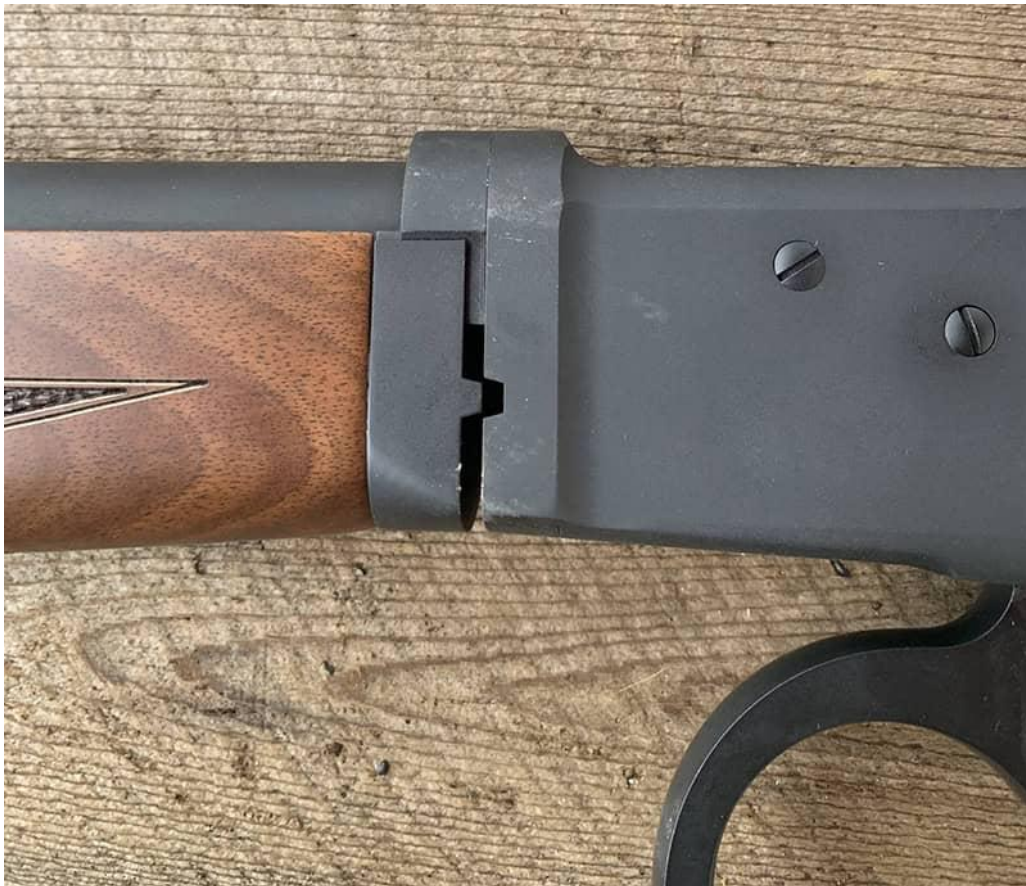
Here's the mortise in open position, ready to be taken down by sliding the halves apart.
