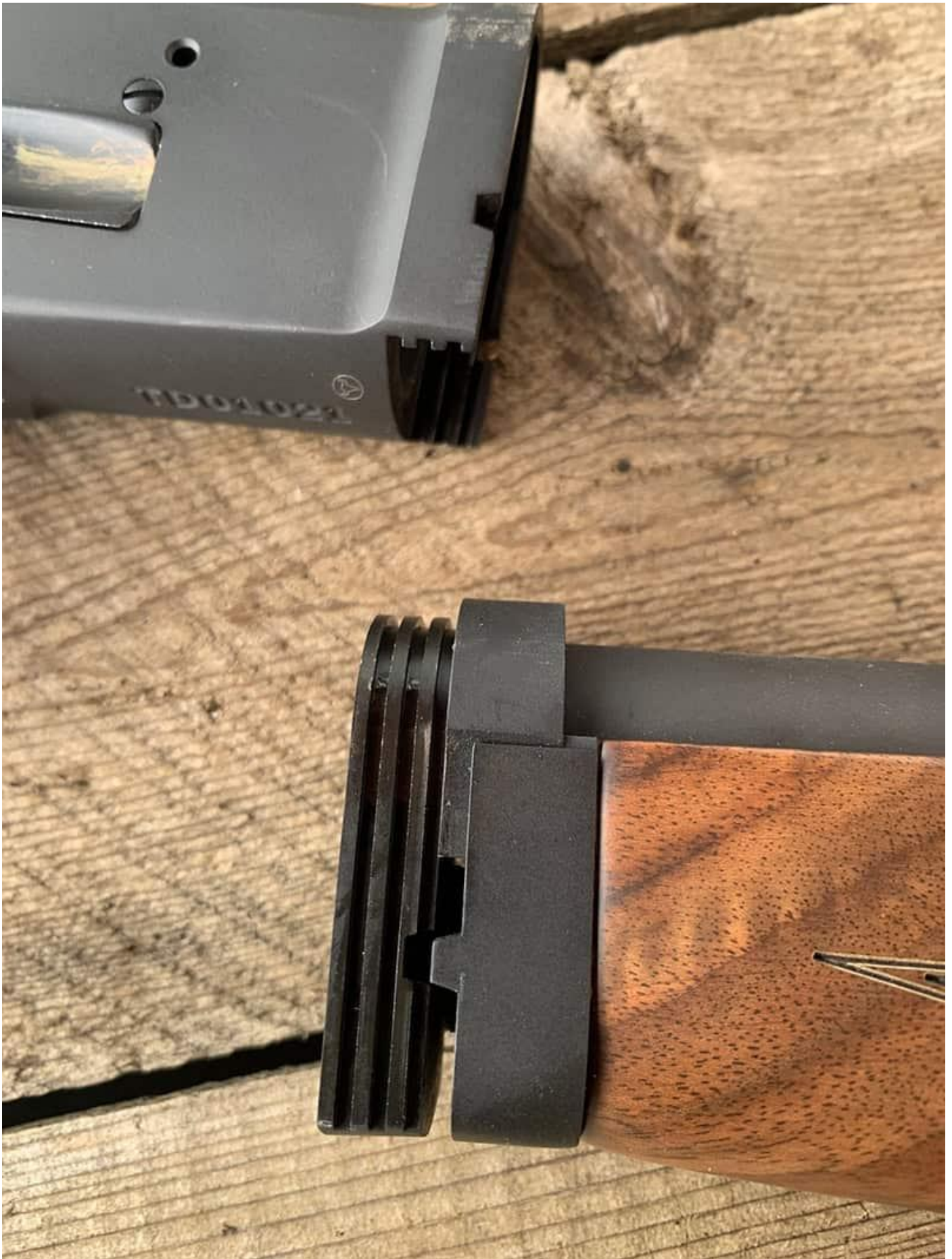
Close-Up of the splines and retracting mortise secure take-down possible.
