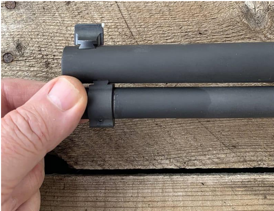
Turning the knurled magazine tube activates the mortise joint.
