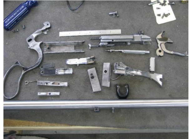
The internal parts of the original Model 89. Note the bottom cover next to the lever.
